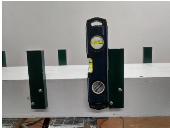
Photo 6. Ensure Station Blocks are Vertical.
